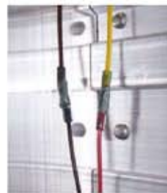
Shrink tubing connectors keep connections secure.
