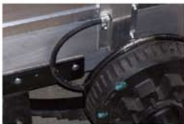
Axle wiring is completely covered.
