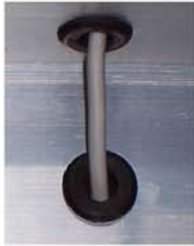
Grommets keep wires from rubbing on the aluminum and being cut.
